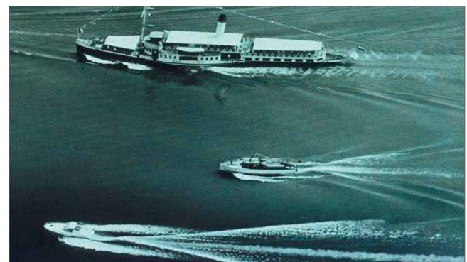
Fig. 4.1.1-17: Secondary waves produced by displacement (vessel right, top and middle) and planing boats at corresponding speeds [BAW]
