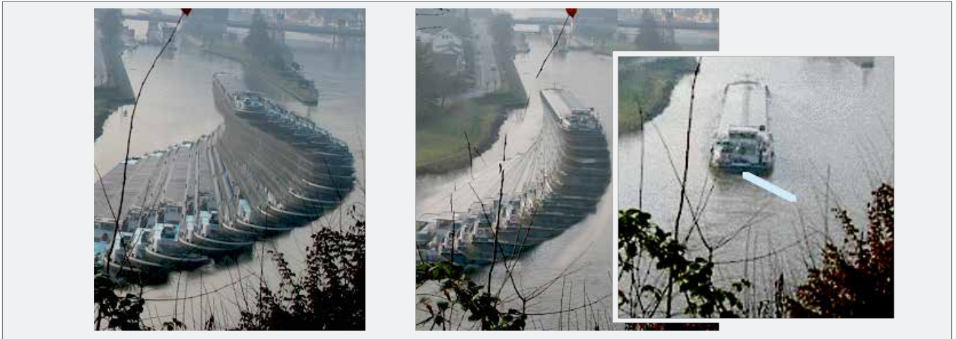
Fig. 4.1.4-1: Two GMSs with good (sailing close to the left bank, early turn into the lay-by basin, photo right) and not-so-good strategies to enter a lock approach (sailing on the outside of the bend and drifting off in the cross flow field, left photo) [BAW]
