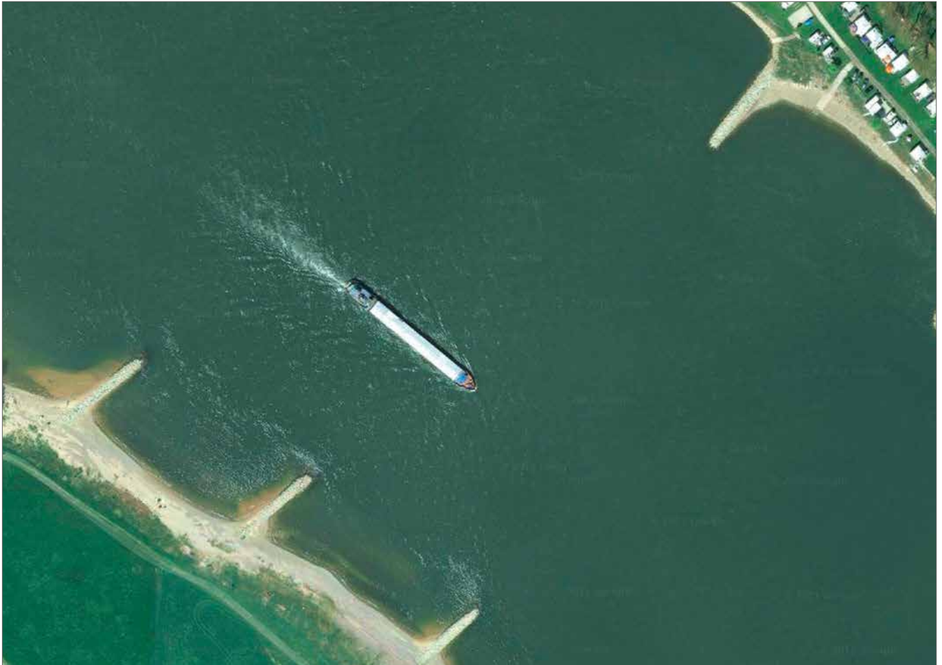
Fig. 4.2.2-1: Inland navigation vessel sailing upstream past a groyne field on the Rhine near Dormagen (the water flows from the bottom of the photograph to the top) [source: Google Maps]
