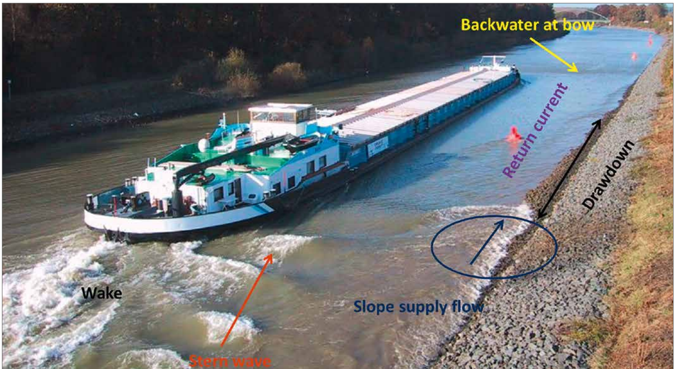
Fig. 4.1.1-1: Ship-induced flows and waves from the primary wave field during displacement motion in a navigation channel of limited width and depth [BAW]
