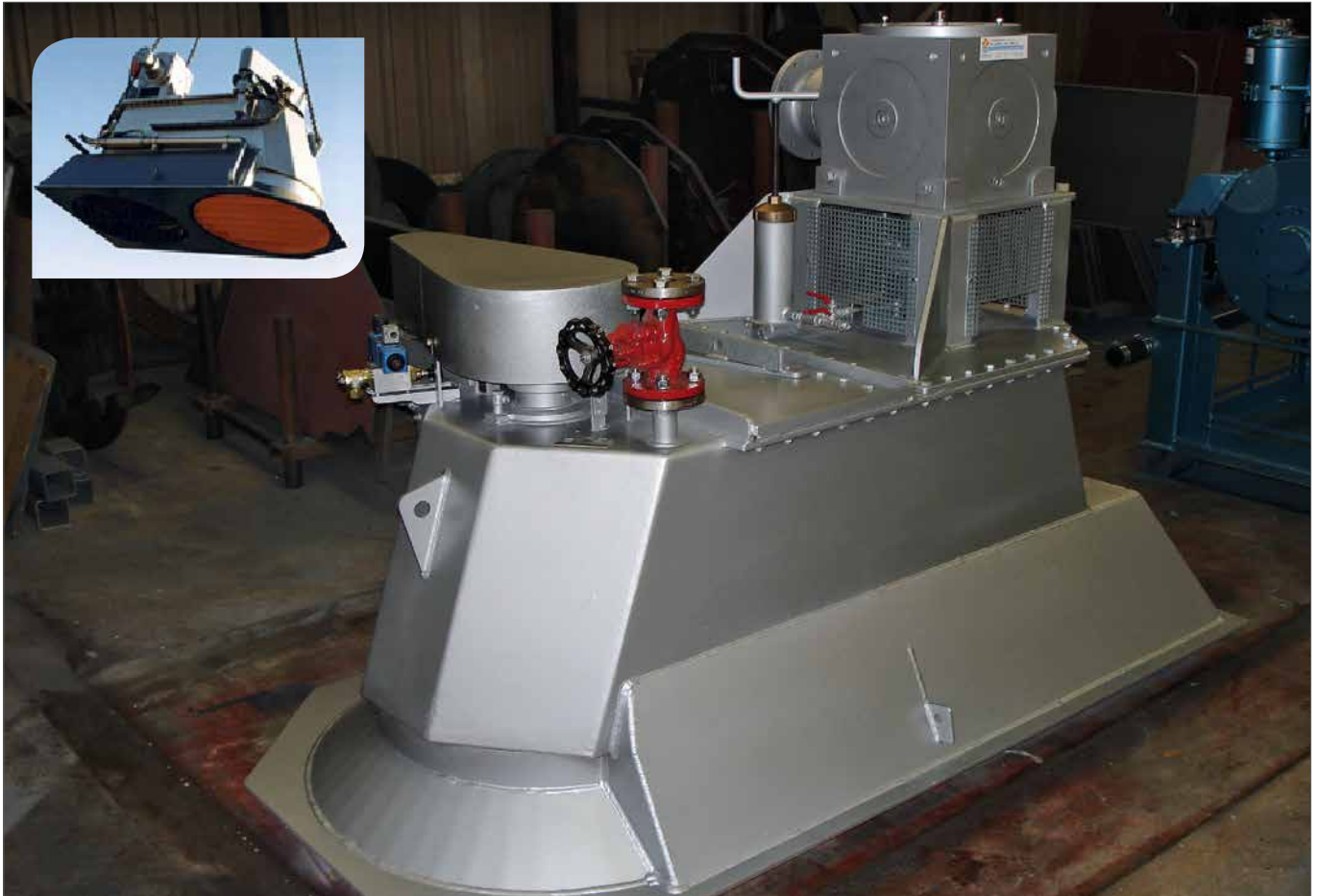
Fig. 2.3.3-2: Bow thruster with propeller in vertical position. Top left: design with a steering grid that can rotate by 360° [Van Tiem, Druiten, Netherlands]
