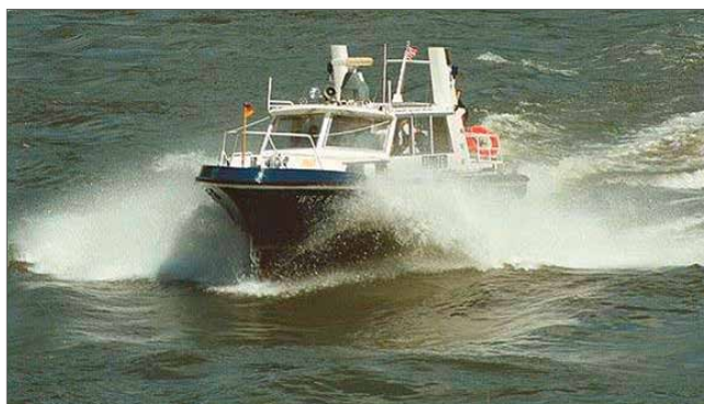
Fig. 4.1.1-17: Secondary waves produced by displacement (vessel right, top and middle) and planing boats at corresponding speeds [BAW]
