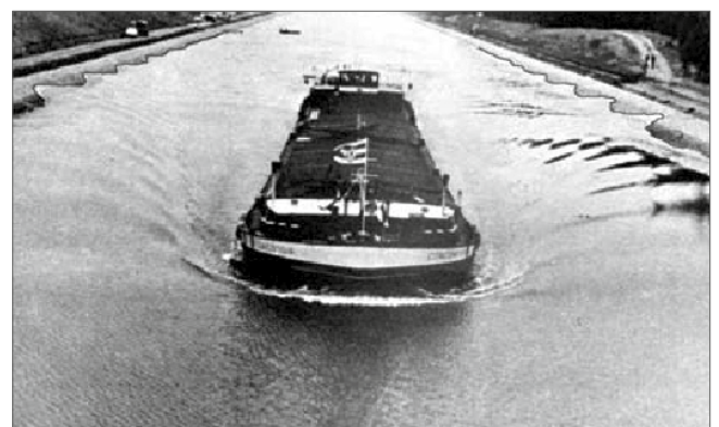
Fig. 4.1.1-14: Conventional Europe ship sailing at 12\text{ km/h} \approx v_{crit} during tests on the Main-Danube Canal (source: GBB, 2004) [VBW/BAW]
