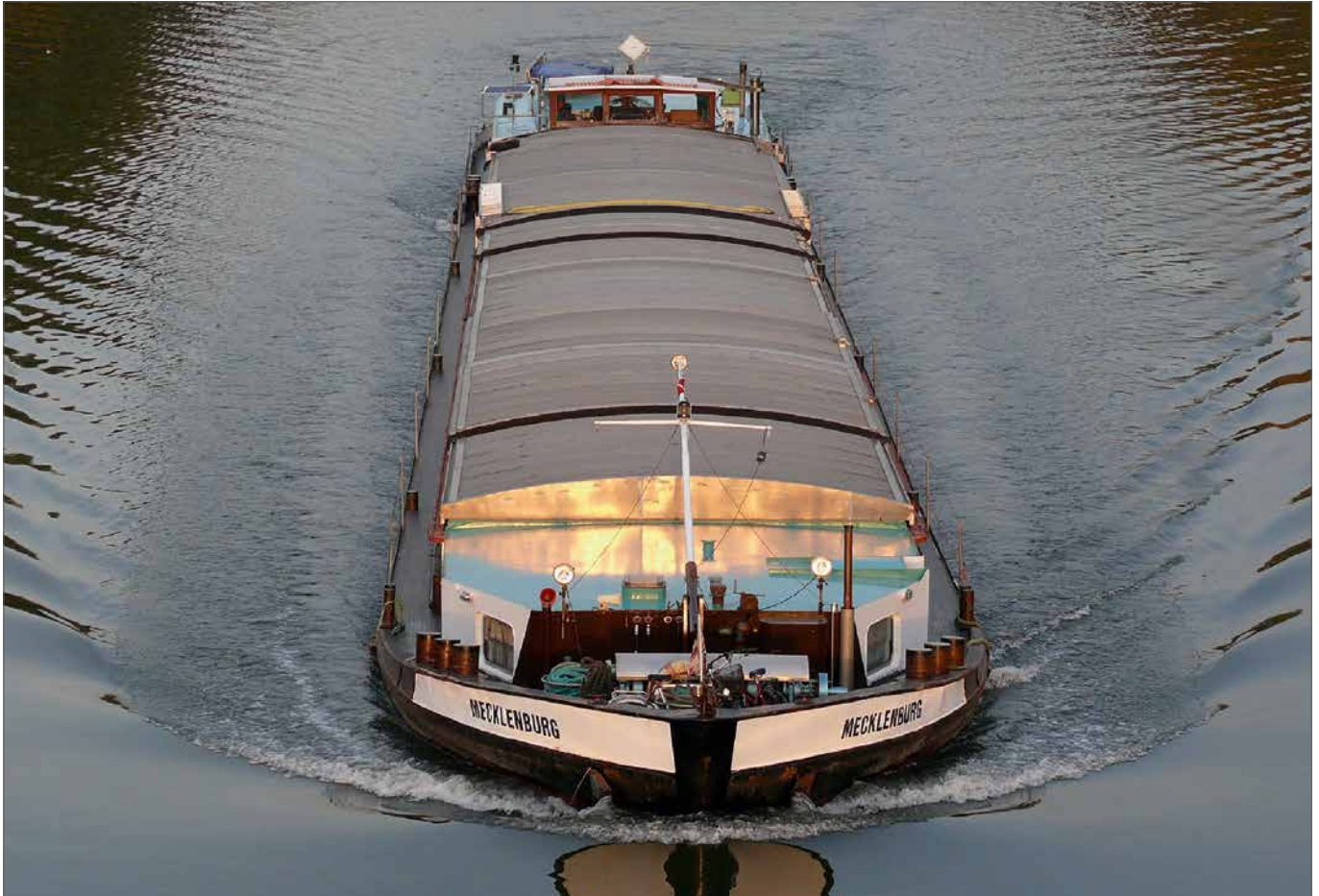
Motor vessel, Gustav Königs – Class III (with dry cargo) [photo: Liebthal, pixelio.de]
