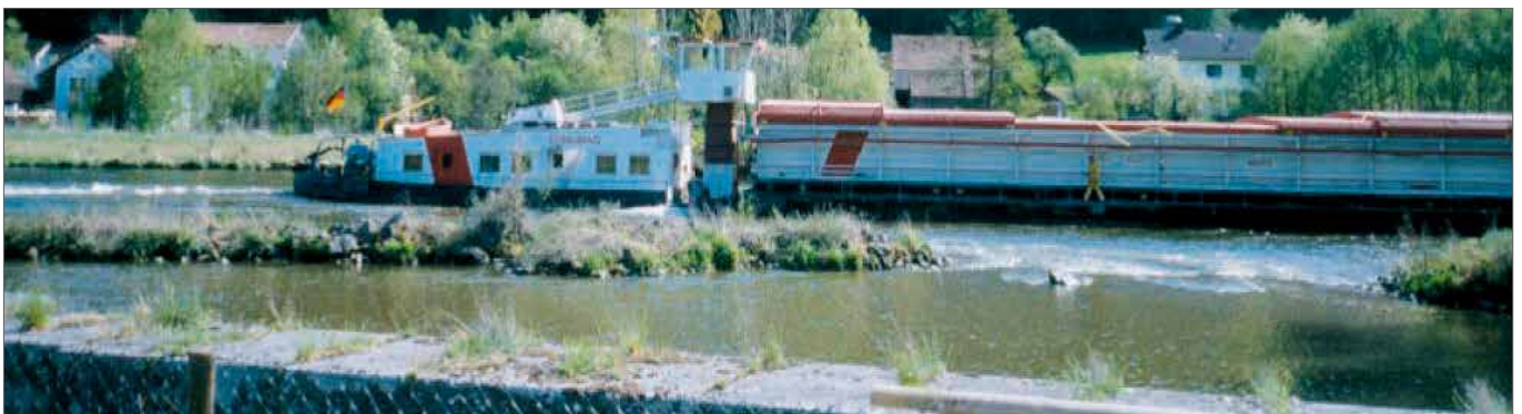
Fig. 4.1.2-1: Pushed convoy on the Main-Danube Canal near Riedenburg. The drawdown is visible from the flow from the bow in the foreground towards the canal [BAW]
