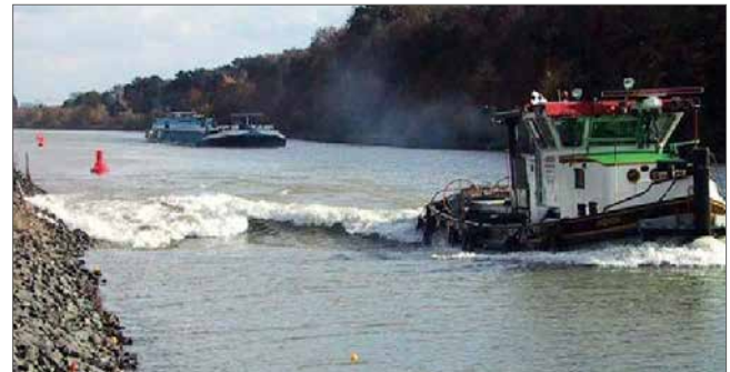
Fig. 4.1.1-16: Superimposed bow and transverse stern waves of a tug boat sailing close to the bank – situation according to Fig. 4.1.1-15 [BAW]
