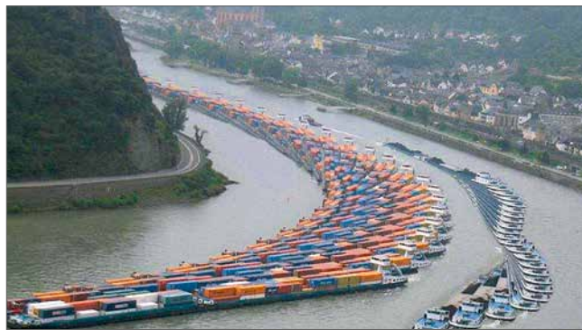
Fig. 4.1.5-1: Container unit (breasted-up formation, GMS and 3 barges, left) sailing downstream in the Rhine near Oberwesel, encountering a towed, single-line pushed convoy with one barge navigating upstream (right) [BAW]
