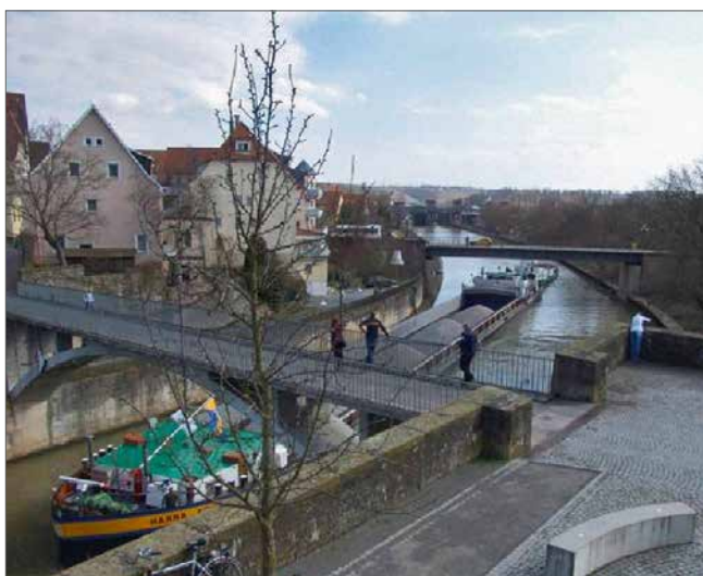
Fig. 4.1.5-14: Field test to simulate navigation of an üGMS past the town of Lauffen (Neckar) with a unit comprised of the push boat Vogel Gryff and the MS Hanna Krieger (overall length: 139 m) [BAW]
