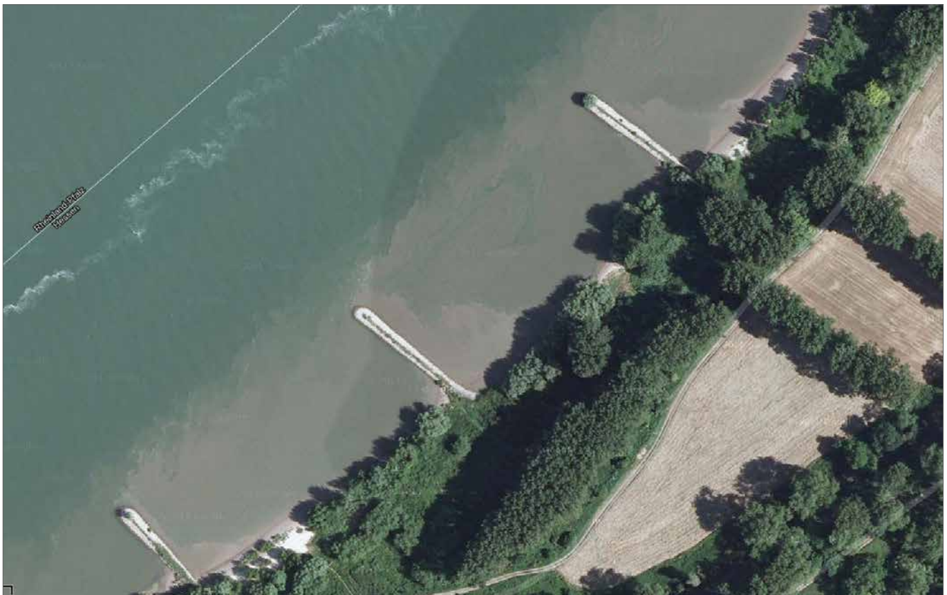
Fig. 4.1.9-1: Right bank of the River Rhine in the groyne field near Biblis: the water flows from the bottom of the photograph to the top [source: Google Maps]
