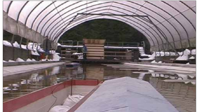
Fig. 4.1.9-4: Breasted-up formation sailing slowly downstream along groyne fields and encountering a GMS in model tests to determine the necessary safety distances at groynes [Neuner, 1999]
