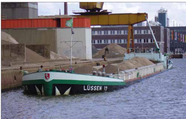
Inland navigation vessel, Johann Welker class with dry cargo [photo: Jan v. Bröckel, pixelio.de]
