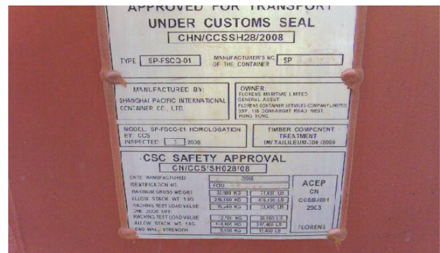
Abb. 2-6: CSC-Schild auf Containerwand [Foto: RRT] Fig. 2-3: Exact height indicated on the container side wall [photo: RRT]
