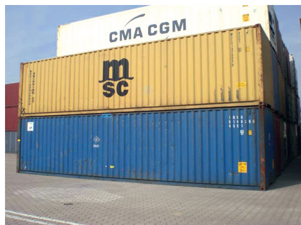
Abb. 2-16: 40' Box High Cube [Foto: VBW] Fig. 2-16: 40' high cube box [photo: VBW]
