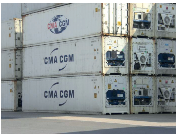
Abb. 2-15: 40' Reefer [Foto: VBW] Fig. 2-15: 40' reefer [photo: VBW]
