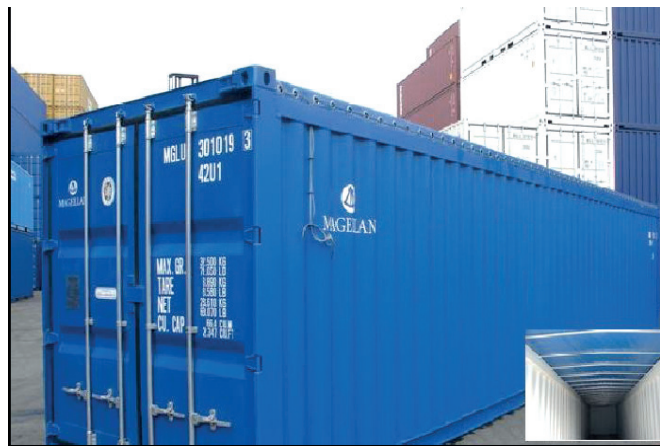
Abb. 2-14: 40' Open Top [Foto: MM] Fig. 2-14: 40' open top [photo: MM]
