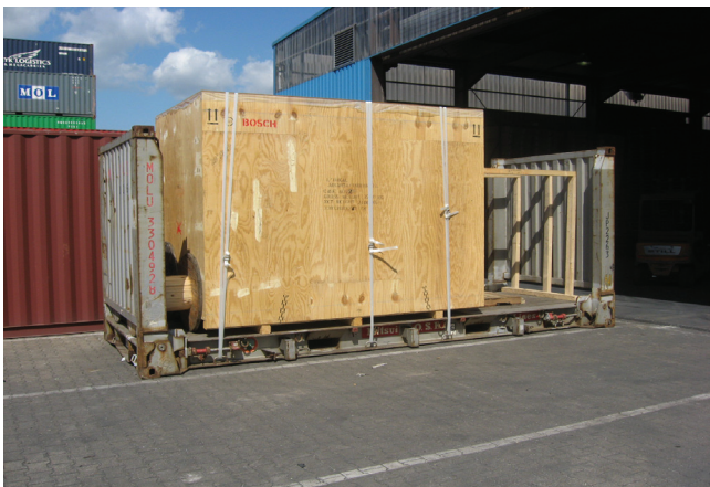
Abb. 2-9: 20' Flat rack [Foto: VBW] Fig. 2-9: 20' flat rack [photo: VBW]
