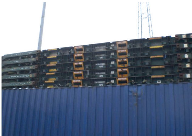
Abb. 2-13: 40' Flat rack [Foto: MM] Fig. 2-13: 40' flat rack [photo: MM]
